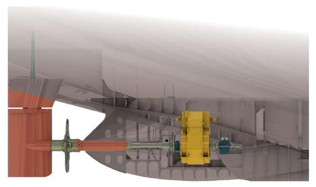
■ The installation features a full variable speed diesel electric package propelled by two fully-feathering controllable-pitch propellers
